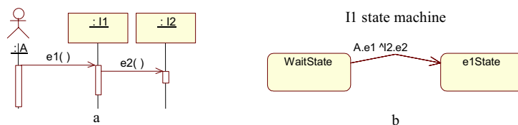
Figure 8. Representation of Received Request Event , having succeeding Sent Request , on sequence diagram (a) and on state machine (b)
